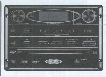
TUNE/TRACK: Rotate UP or DOWN to adjust HOUR and MINUTES once in CLOCK MODE or ALARM SETTING MODE.
