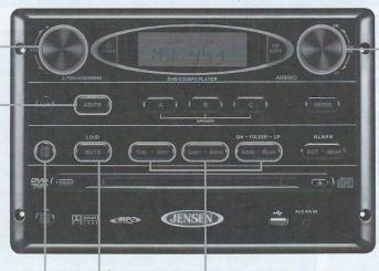
TUNE/TRACK: Rotate counter-clockwise to TUNE DOWN in frequency in AM or FM Mode. Rotate clockwise to TUNE UP in frequency AM or FM Mode. Rotate and hold to scan to next strongest station.
